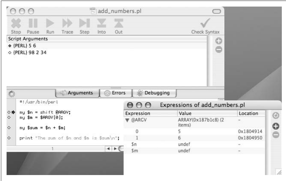
Figure 4-6. Affrus allows me to configure several different command lines to use with my program; it updates expressions as my program runs
